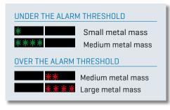
Green and Red Metering Signals Proportional to the Metal Mass Detected
